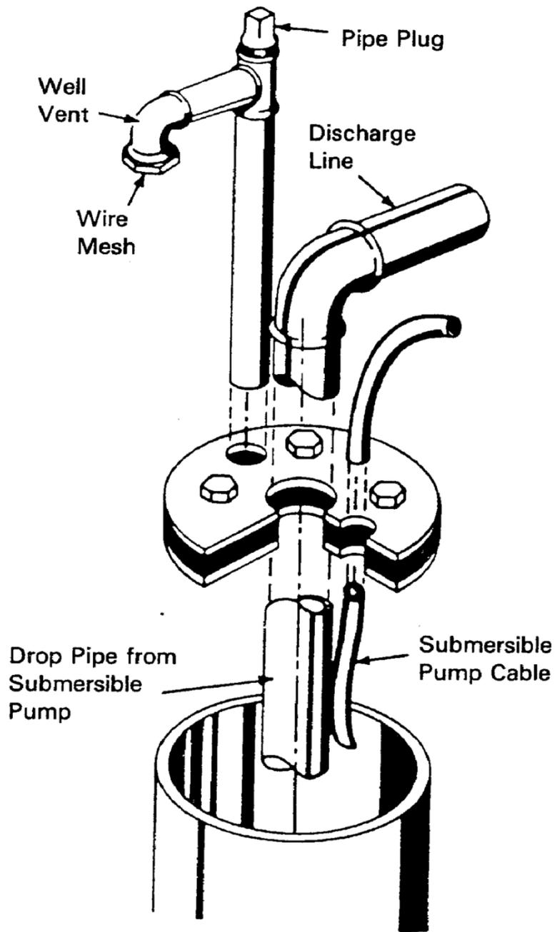
Figure 27. Well Seal for Submersible Pump Installation
