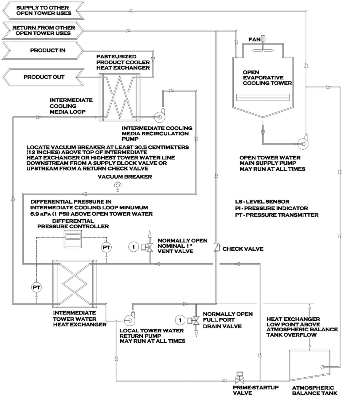
① THIS VALVE MUST AUTOMATICALLY OPEN AND REMAIN OPEN WHENEVER THE REQUIRED PRESSURE DIFFERENTIAL IN THE INTERMEDIATE TOWER WATER HEAT EXCHANGER DOES NOT EXIST.
